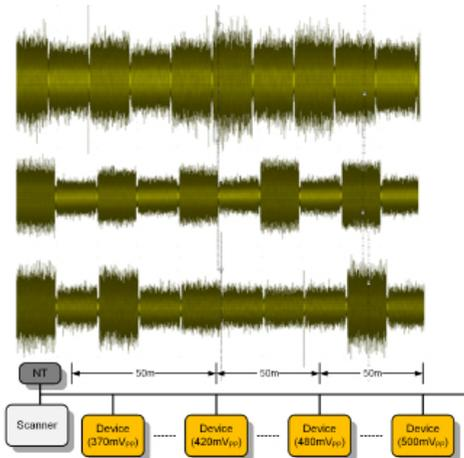
Figure 20: Impact of signal level and network position
