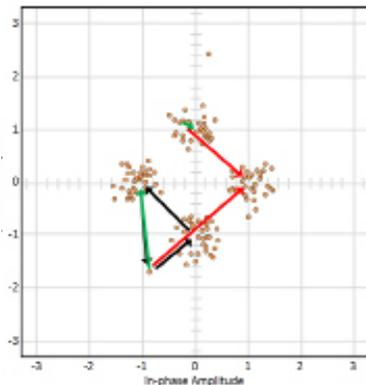
**Decoding:** Ideal signal pulses are sent and impacted by noise.
