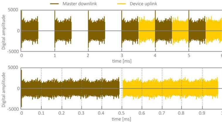
Figure 18: Device synchronization with the master signal
